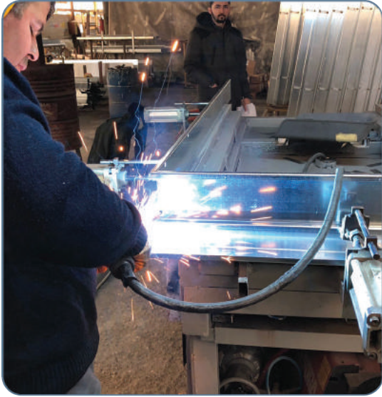
Corner 45° Argon welding Detail
