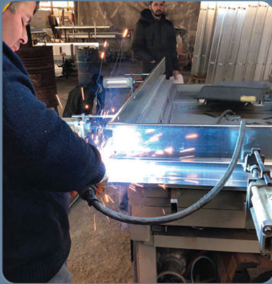
Corner 45° Argon welding Detail
