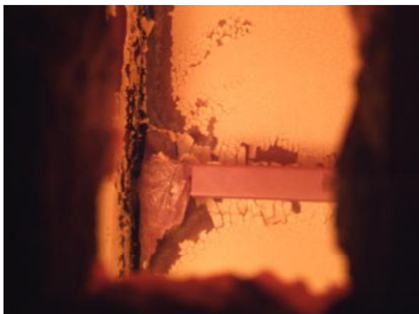
15 th minute of the test Exposed door face – lock.
