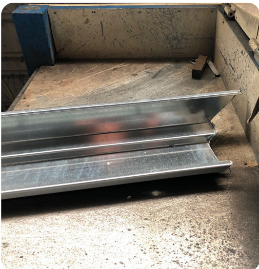
The Joints Of The Cases Are Cut At 45 Degrees
