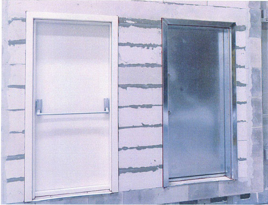
Photo C2: Exposed side of the test specimens before the test.
