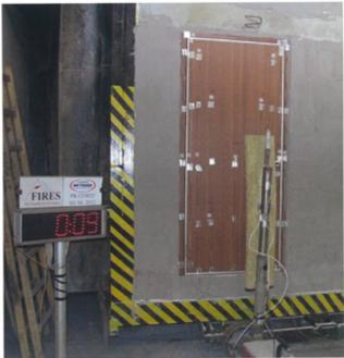
Unexposed specimen face before the test commencement
