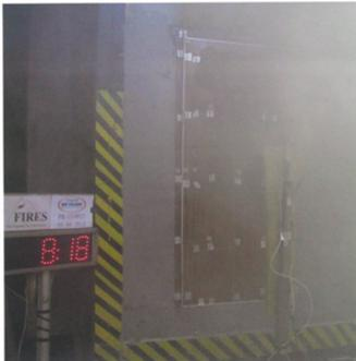
3<sup>rd</sup> minute of the test Smoke release around the perimeter of door leaf.
