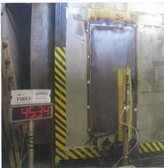
32<sup>nd</sup> minute of the test Door leaf surface treatment is completely fallen down.
